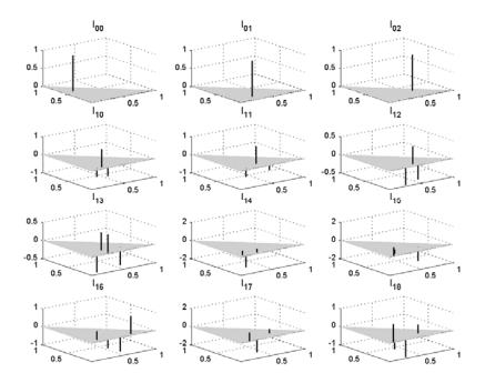
FIGURE 2.3. Collocation functionals in  $L_0$  and  $L_1$  on the unit triangle.
