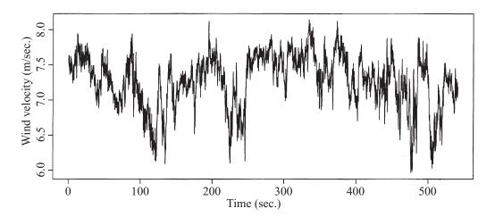
Figure 2. Streamwise wind velocity component in metres per second plotted against time in seconds.
