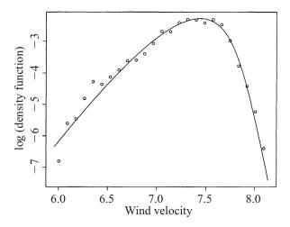
Figure 4. Log histogram of the wind velocity data with a fitted variance-gamma log-density function.
