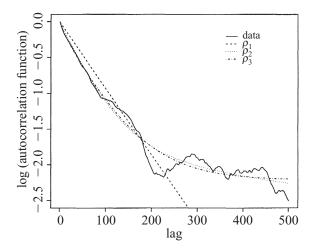
**Figure 6.** The log empirical autocorrelation function of the wind velocity data with fitted curves corresponding to the logarithm of one, two, and three exponential functions.
