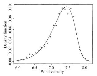
Figure 3. Histogram of the wind velocity data with a fitted variance-gamma density function
