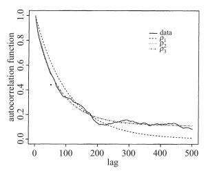
Figure 5. The empirical autocorrelation function of the wind velocity data with fitted curves corresponding to one, two, and three exponential functions.
