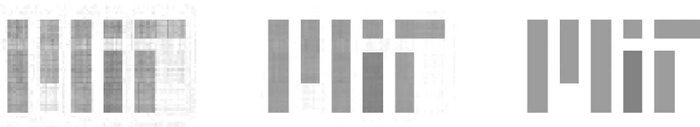
FIG. 7. Recovery of MIT logo based on different number of measurements. Left: 900; Middle: 1000; Right: 1080.
