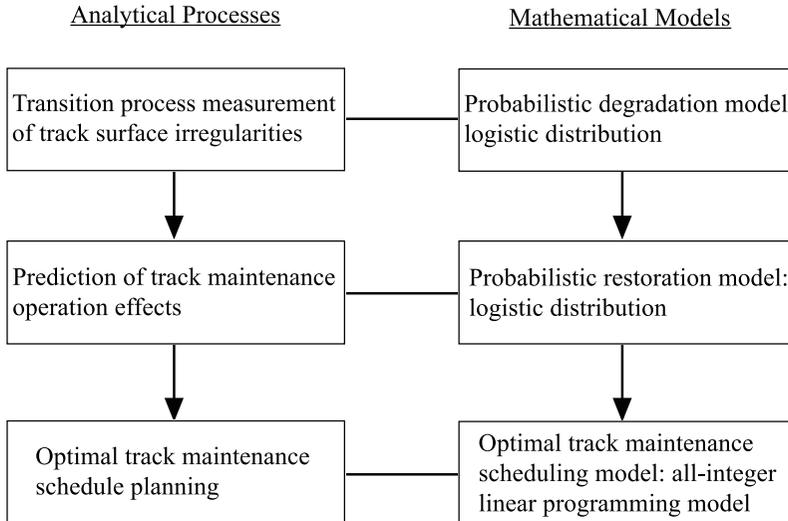
Fig. 1. Flow diagram of the computational procedures.
