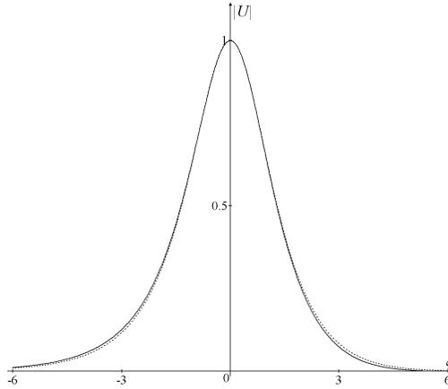
Figure 3. The numerical result (the solid curve) for the soliton's envelope,  $|U(\xi)|$ , within the time interval  $5 < t \leq 400$  for  $\mu = 5/48 \equiv \mu_*$  (evidently, the soliton keeps the established shape in the course of this interval of time). The dotted curve shows the profile of the analytical solution (4.1) (see the text).
