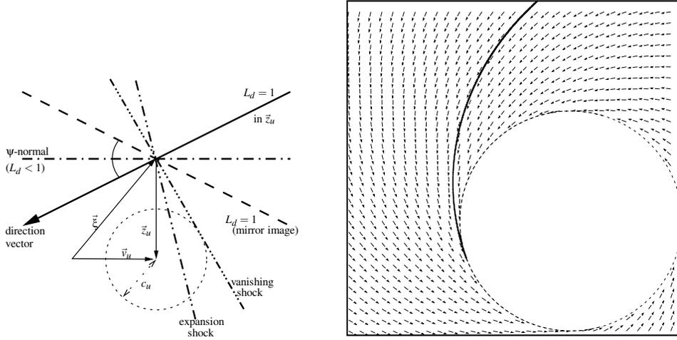
Figure 8. Left: through each  $\vec{\xi}$  farther than  $c_u$  from  $\vec{v}_u$  there are exactly two straight shocks (solid, dashed) with  $L_d = 1$ , mirror images of each other. The shocks with  $L_d \leq 1$  are between them (indicated by arc left of  $\vec{\xi}$ ). The solid lines define the direction field whose integral curves are “envelopes”. Right: no shock with  $L_d \leq 1$  can approach  $\vec{v}_u$  faster (in counterclockwise direction) than the counterclockwise envelope.
