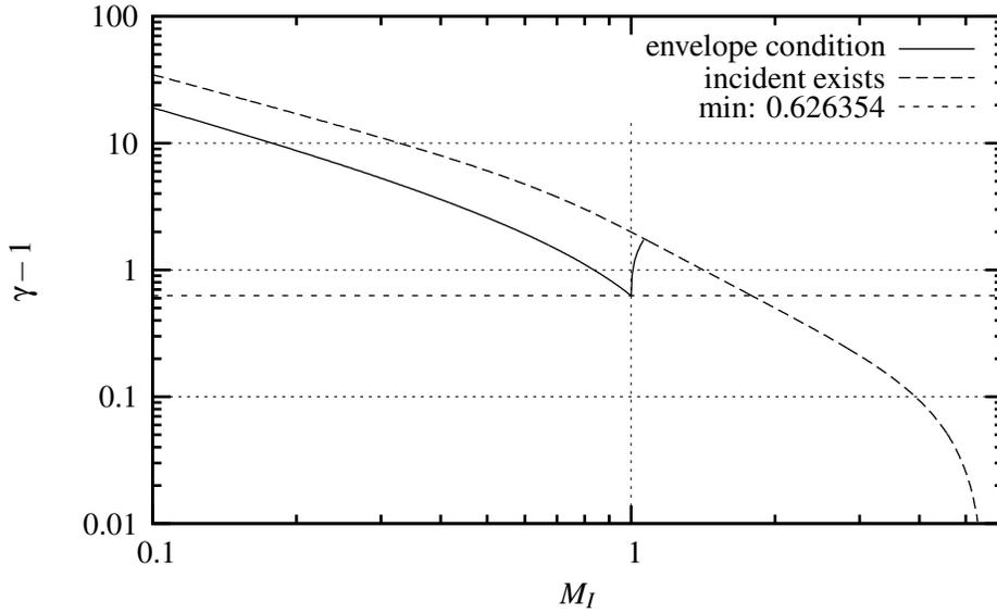
Figure 9. For  $\beta_Q = 0$  (vertical incident shocks) and the set of  $M_I, \gamma$  enclosed below the dashed and above the solid line, solutions can be constructed for all  $\theta \in (\theta_s, \frac{\pi}{2}]$ .
