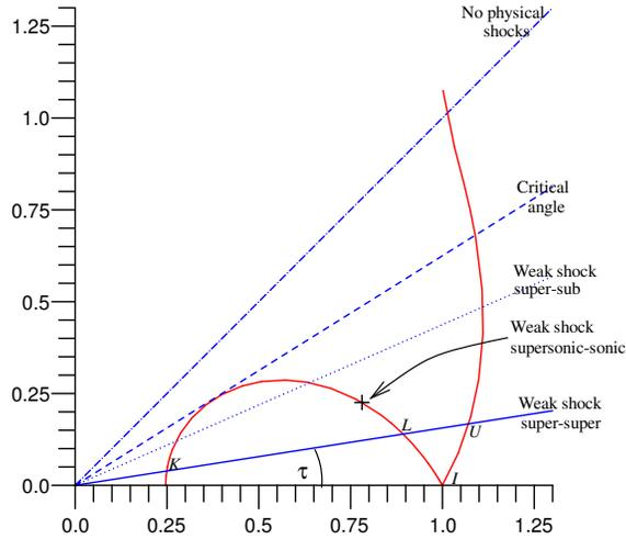
Figure 2. A given upstream velocity ( $I$ ) with possible downstream velocities (red curve) for steady shocks with varying normal. The  $U$  shock is unphysical;  $K$  is the strong and  $L$  the weak shock. Shocks cannot turn velocities by more than the critical angle  $\tau_*$ .
