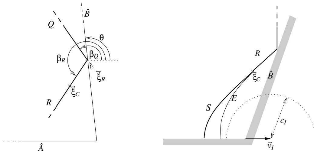
Figure 6. Left: a local RR pattern; right: the curved portion  $S$  of the reflected shock has  $L_d \leq 1$ , hence must be left of the envelope  $E$ , which bounds it away from the dotted circle and from  $\hat{B}$ .
