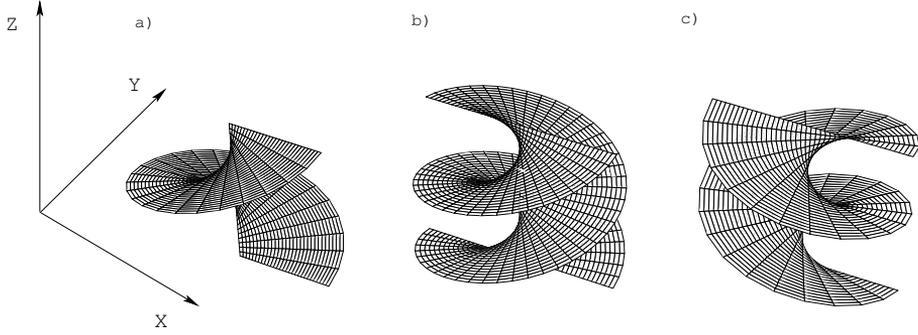
Figure 4: Helicoidal structures of wavefront around  $\tau$ -axis: a) one-start right-screw ( $K = 1$ ); b) two-start right screw ( $K = 1$ ); c) two-start left screw ( $K = -1$ ).
