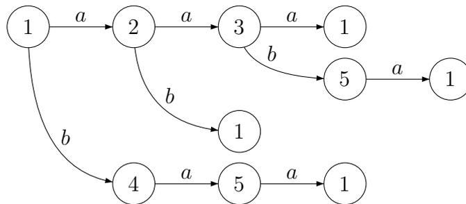
Figure 2: The minimal automaton of  $\{aaa, aaba, ab, baa\}^*$
