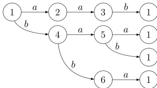
Figure 7: The minimal automaton of  $\{aab, baa, bab, bba\}^*$
