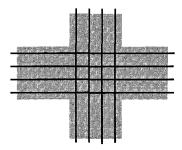
FIGURE 9. Manhattan: crossing of the box with 4 by 4 strands.
