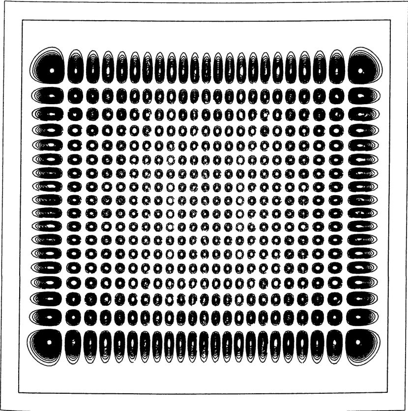
Figure I. Transverse Eigenmodes of a Rectangular Laser. Computer Plot.
