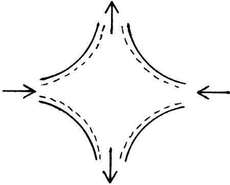
Figure 4. Sketch of boundaries of a rheometer. Arrows show flow direction of a viscous test fluid. A less viscous lubricant flows next to the walls.
