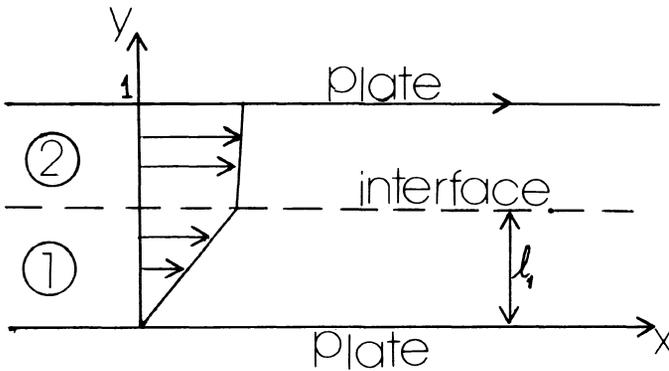
Figure 5. Undisturbed two-layer flow. Fluid 1 occupies  $0 \leq y \leq l_1$ . Fluid 2 occupies  $l_1 \leq y \leq 1$ . The fluids have viscosities  $\mu_i$  ( $i = 1, 2$ ) and densities  $\rho_i$ . Upper plate speed is 1.
