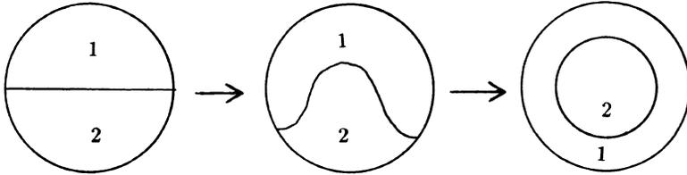
Figure 1. Evolution of flat interface into the encapsulated arrangement
