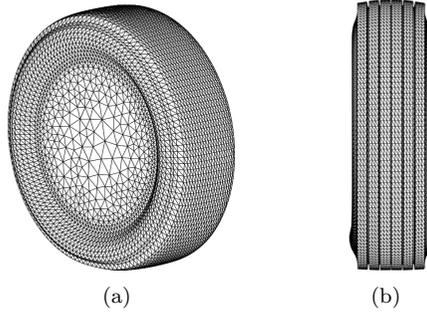
FIGURE 6. Discretization of car, respectively, truck, tires used for computations [16].
