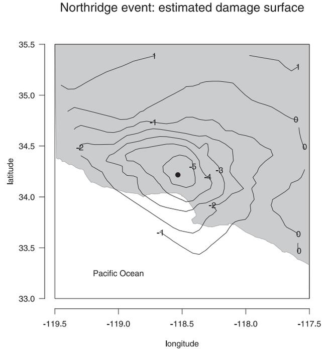
FIG. 4. The estimate of the function  $f_{x,y}$  of (2). The smaller the contour level, the greater the damage.
