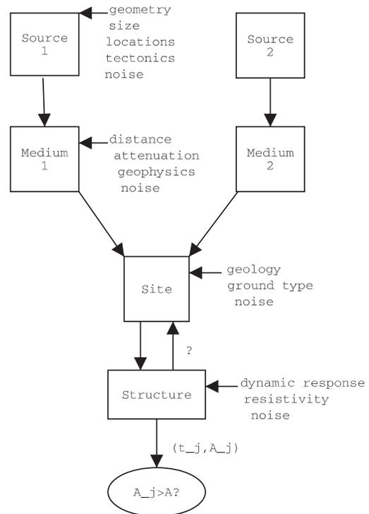
FIG. 2. Box-and-arrow diagram highlighting components of seismic risk analysis. The symbol  $A_j$  refers to the level of some performance variate associated with the  $j$ th event;  $A$  is a threshold level.
