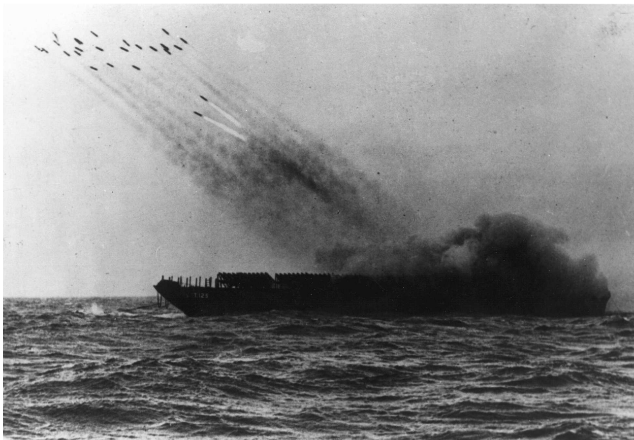
FIG. 1. An LCT(R) [Landing Craft Tank (Rockets)] firing 5-inch rockets in training for D-Day. Picture, Imperial War Museum.
