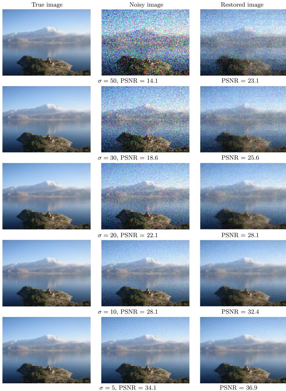
Fig. 2. The result of the experiment on image denoising. Left: the original  $120 \times 160 \times 3$  image. Middle: the noisy image for different values of  $\sigma$ . Right: the denoised image.
