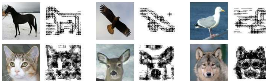
FIG 2. Real images and their binary sketches. Each bar in the sketch image indicates the existence of a Gabor filter response above a threshold within a local cell of the image.
