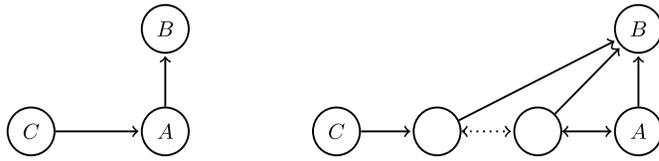
FIG. 1. Edge configurations in MAGs and PAGs for a visible edge  $A \rightarrow B$ ; cf. Zhang (2008a), Figure 6. Instead of the tail mark at  $C$ , one can also have an arrowhead or circle mark.
