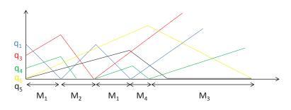
FIG 4. A fluid limit sample path for the broken-diamond network of Figure 3, corresponding to the switching sequence  $M_1 \to M_2 \to M_1 \to M_4 \to M_3$ .
