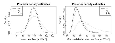
FIG. 7. Estimated posterior densities of the means,  $v_D$  and  $v_S$  (left), and the standard deviations,  $\tau_D$  and  $\tau_S$  (right), of the background heat flow for both regions. The (marginal) prior distributions are the same for both regions and are presented with dotted lines.
