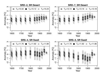
FIG. 9. Comparison of posterior distributions of GST histories for 4 boreholes using different values for the temperature intercept  $T_{0j}$ . The white squares show the estimated posterior means and the vertical bars show the symmetric 50% (thick) and 90% (thin) posterior credible intervals. At each time point the middle bar shows the original results (same as in Figure 2) and the left and right bars show the results for lower and higher values of  $T_{0j}$ , respectively.
