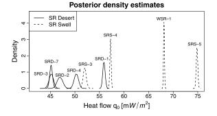
FIG. 6. Estimated posterior densities of the heat flow  $q_{0j}$  for boreholes from the San Rafael Desert (solid lines) and San Rafael Swell (long dashes).
