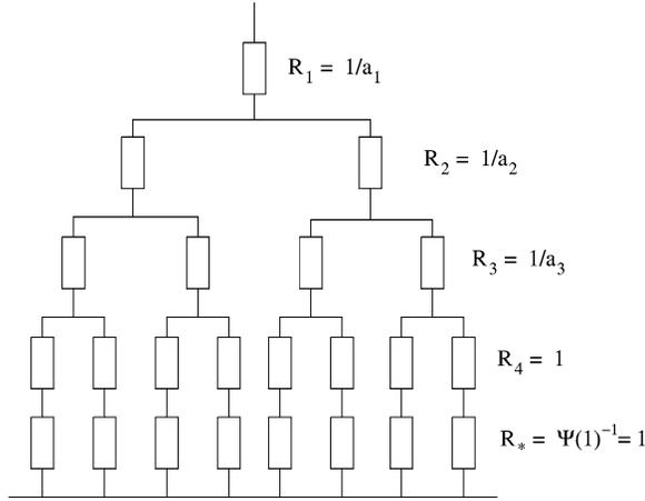
FIG. 5. *Tree-structured resistor network identified with the attribute hierarchy, where  $a_l = \Gamma(|A_l|)$  is the complexity of attributes of level  $l$  and  $R_l = 1/a_l$  is the associated resistance; note that  $a_4 = 1$  by convention for the bottom attributes. The last row of resistors represents the postprocessing stage. The conductance of this circuit is exactly the CTF testing cost of the attribute hierarchy when  $\Psi$  is the harmonic power function.*
