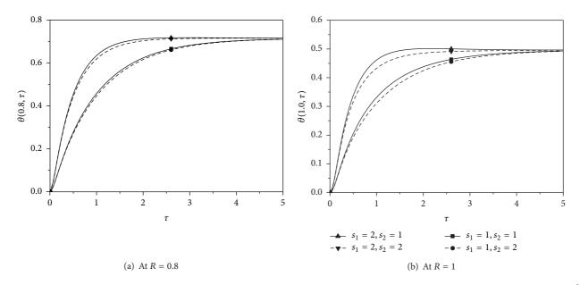
FIGURE 3: Influence of function parameters  $s_1$  and  $s_2$  on the temperatures of the hollow cylinder at middle and right surfaces,  $[\psi(\tau) = 1 - e^{-s_1\tau}, Bi(\tau) = 2 - e^{-s_2\tau}, \overline{\theta}_0 = 0]$ .
