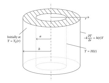
FIGURE 1: Hollow cylinders with time-dependent temperature and time-dependent heat transfer coefficient at inner and outer surfaces.
