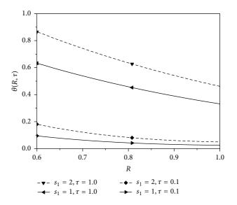
FIGURE 2: Temperature distribution and variation along the radial of the hollow cylinder with different parameter  $s_1$  of temperature function  $\psi(\tau)$ ,  $[\psi(\tau) = 1 - e^{-s_1\tau}$ ,  $\operatorname{Bi}(\tau) = 2 - e^{-\tau}$ ,  $\overline{\Theta}_0 = 0]$ .
