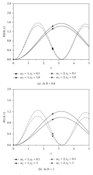
FIGURE 5: Influence of  $\omega_1$  parameter and  $s_2$  parameter on the temperature variation of the hollow cylinder at middle and right surfaces,  $[\psi(\tau) = 1 - \cos \omega_1 \tau, \operatorname{Bi}(\tau) = 2 - e^{-s_2 \tau}, \overline{\theta}_0 = 0]$ .
