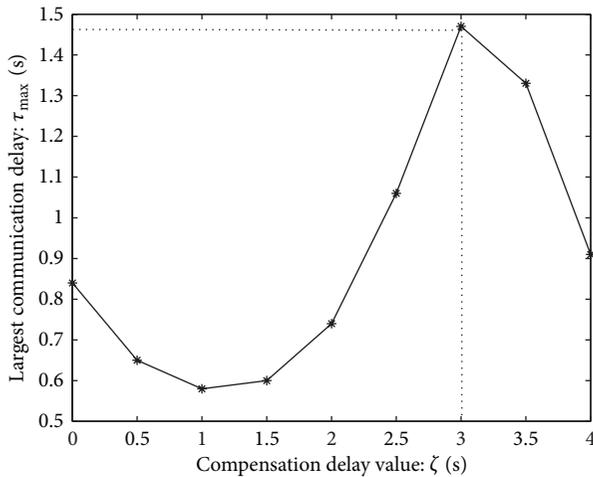
FIGURE 6: Bound of communication delay with different  $\zeta$ .
