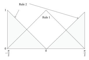
FIGURE 1: Membership functions of two-rule model.
