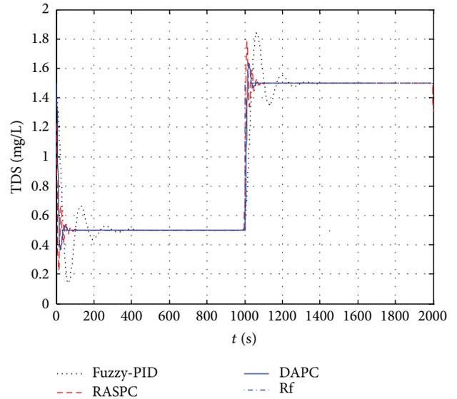
FIGURE 5: The tracking comparison of output TDS.
