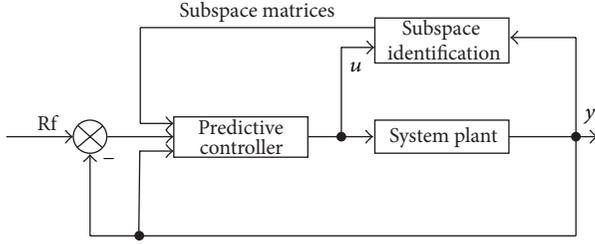
FIGURE 1: The structure of closed-loop data-driven predictive control.
