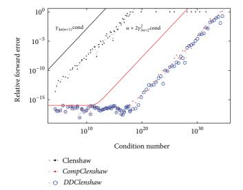
FIGURE 3: Accuracy of evaluation of polynomial converted from  $p(x) = (x-0.75)^7 (x-1)^{11}$  by the *DDConvert* algorithm in Legendre basis with respect to the condition number.
