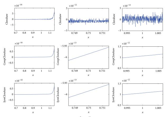
FIGURE 1: Evaluation of polynomial converted from  $p(x) = (x-0.75)^7 (x-1)^{11}$  by the *Convert* algorithm in Legendre basis in the neighborhood of its multiple roots, using the Clenshaw algorithm (up), the *CompClenshaw* algorithm (middle), and Symbolic Toolbox (down).
