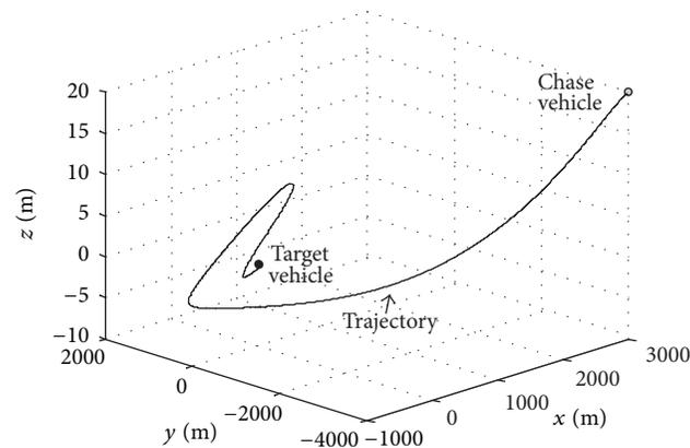
FIGURE 5: Rendezvous trajectory of the chase vehicle.
