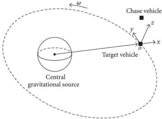
FIGURE 1: Relative Cartesian coordinate system for spacecraft rendezvous.
