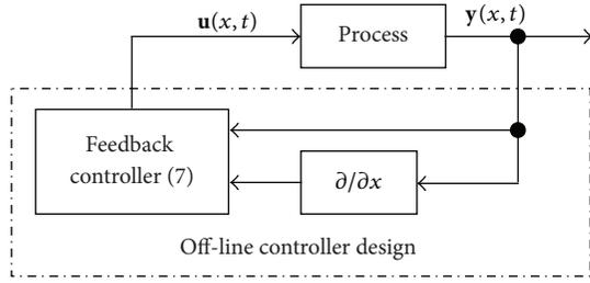
FIGURE 1: The structure of distributed P-sD state-feedback controller.
