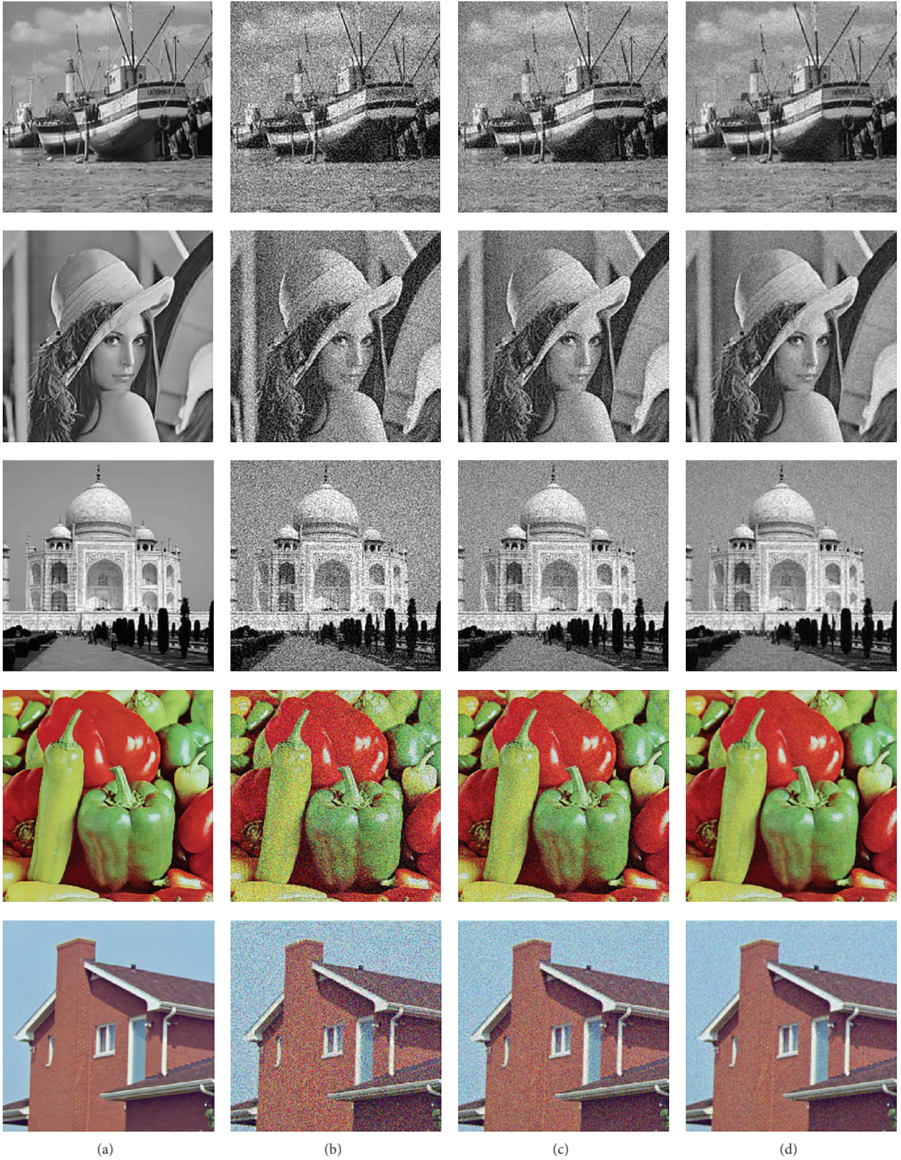
FIGURE 6: Denoising results, (a) original image, (b) corrupted image with additive white Gaussian noise with \sigma value of 25, (c) Gaussian smoothing filter, and (d) FHD filter.
