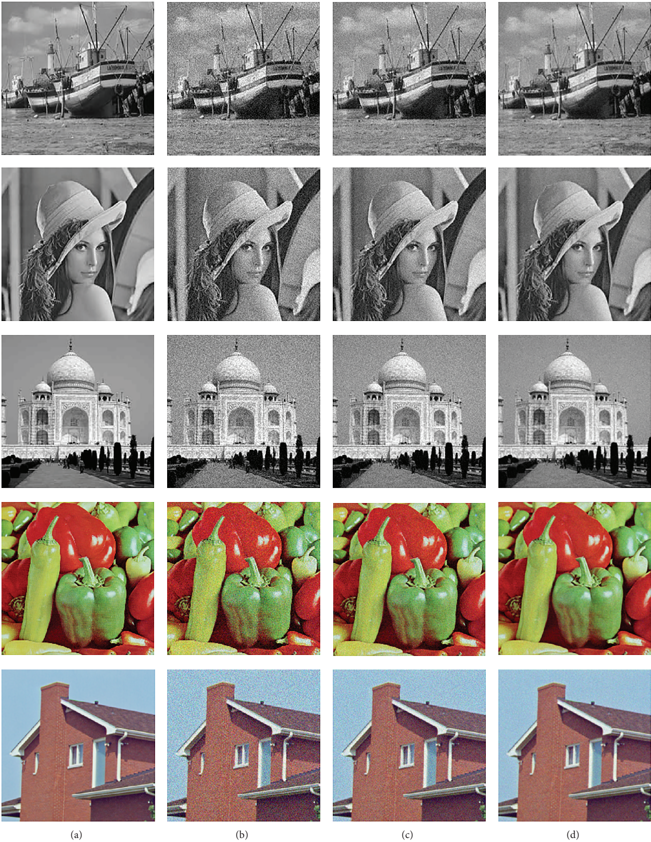
FIGURE 5: Denoising results, (a) original image, (b) corrupted image with Gaussian noise with \sigma value of 15, (c) Gaussian smoothing filter, and (d) FHD filter.
