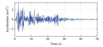
FIGURE 2: Full scale North-South El Centro 1940 seismic record.
