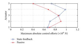
FIGURE 6: Maximum absolute control efforts corresponding to the ideal state-feedback energy-to-peak controller defined by the gain matrix  $\widetilde{G}_s$  (blue line with circles) and the passive-damping system defined by the gain matrix  $\widetilde{K}_d$  (red line with asterisks). The full scale North-South El Centro 1940 seismic record has been used as ground acceleration disturbance.
