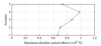
FIGURE 4: Maximum absolute control efforts corresponding to the controlled building with the ideal state-feedback energy-to-peak controller defined by the gain matrix  $\widetilde{G}_s$ . The full scale North-South El Centro 1940 seismic record has been used as ground acceleration disturbance.
