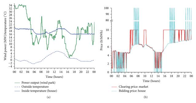
FIGURE 7: Controlled behaviour of an individual house over a 24-hour period in response to varying wind power. (a) Indoor house temperature following wind power. (b) Variation of market clearing price and resulting turning off of loads as a result of changes in wind power (reproduced from Broeer et al. [35] with permission form Elsevier).
