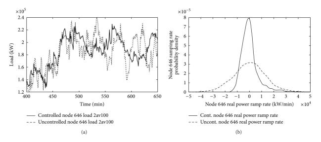
FIGURE 6: Effect of control on (a) load and (b) real power ramp rate (reproduced from [36] with permission from Elsevier).
