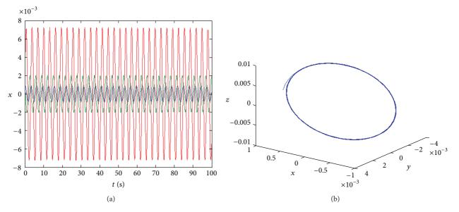
FIGURE 4: Time history and phase diagram of system (3) with a = -1, b = 1, c = -1, e = 18, and d = -0.555556.
