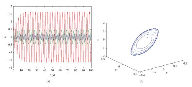
FIGURE 5: Time history and phase diagram of system (3) with a = -1, b = 1, c = -1, e = 18, and d = -0.8.
