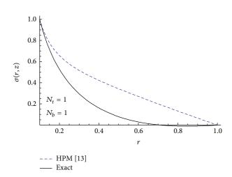
FIGURE 15: Comparison between the HPM and the exact solution for  $\sigma$  at  $N_t = 1$ ,  $N_b = 1$ ,  $r_1 = 0.1$ ,  $\phi = 0.2$ , and z = 0.5.
