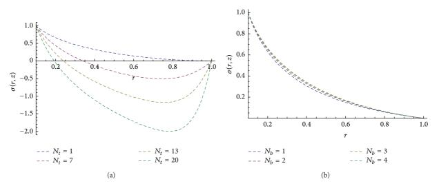
FIGURE 3: (a) Concentration profile for different values of  $N_t$  at  $N_b = 8$ ,  $r_1 = 0.1$ ,  $\phi = 0.2$ , and z = 0.5. (b) Concentration profile for different values of  $N_b$  at  $N_t = 0.5$ ,  $r_1 = 0.1$ ,  $\phi = 0.2$ , and z = 0.5.
