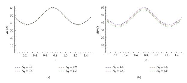
FIGURE 19: Effect of  $N_t$  on pressure gradient for  $r_1 = 0.05$ ;  $\phi = 0.05$ ; Q = -2;  $G_r = 0.3$ ;  $B_r = 0.2$ ;  $N_b = 0.3$ .
