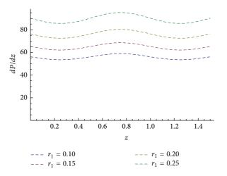
FIGURE 20: Effect of  $r_1$  on pressure gradient for  $\phi = 0.01$ ; Q = -2;  $G_r = 0.3$ ;  $B_r = 0.2$ ;  $N_b = 0.3$ ;  $N_t = 0.3$ .
