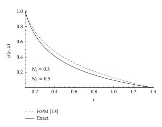
FIGURE 16: Comparison between the HPM and the exact solution for  $\sigma$  at  $N_t = 0.3$ ,  $N_b = 0.5$ ,  $r_1 = 0.1$ ,  $\phi = 0.4$ , and z = 0.3.
