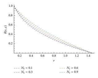
FIGURE 6: Temperature profile for different values of  $N_t$  at  $N_b = 0.5$ ,  $r_1 = 0.1$ ,  $\phi = 0.5$ , and z = 0.3.
