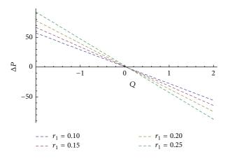
FIGURE 23: Effect of  $r_1$  on pressure rise for  $\phi = 0.05$ ;  $G_r = 0.3$ ;  $B_r = 0.2$ ;  $N_t = 15$ ;  $N_b = 10$ .
