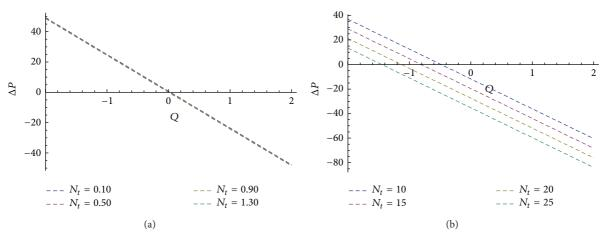
FIGURE 22: Effect of  $N_t$  on pressure rise for  $r_1 = 0.05$ ;  $\phi = 0.05$ ;  $G_r = 0.3$ ;  $B_r = 0.2$ ;  $N_h = 0.3$ .
