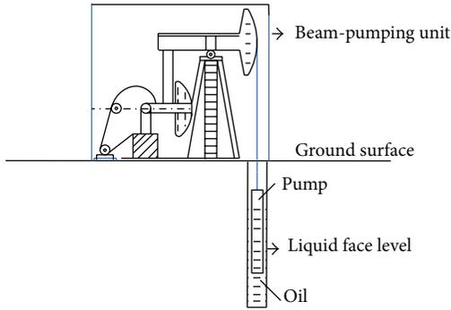
FIGURE 1: The schematic diagram of beam pumping system.
