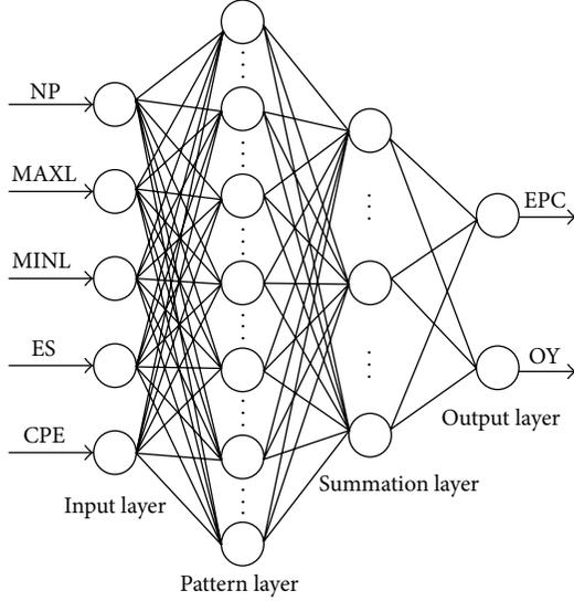
FIGURE 2: GRNN model of the beam pumping system.
