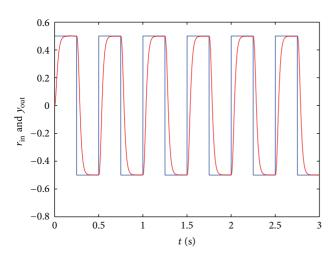
FIGURE 2: Square signal tracking curve of compound control.
