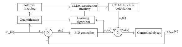
FIGURE 1: The structure diagram of self-tuning parameter PID controller based on CMAC.
