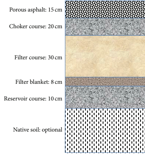
FIGURE 1: Typical cross-section for pervious pavement system.
