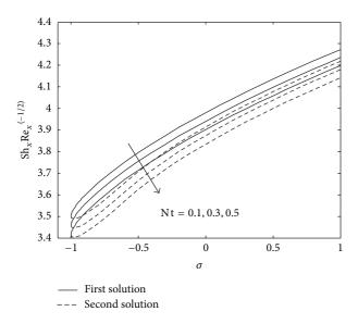
FIGURE 6: Variations of the local Sherwood number (concentration rates) with  $\sigma$  for different values of Nt when Nb = 0.5, Le = 2, Pr = 6.8,  $\gamma$  = 0.1, and *S* = 2.
