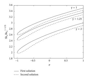
FIGURE 5: Variations of the local Sherwood number (concentration rates) with  $\sigma$  for different values of  $\gamma$  when Nb = Nt = 0.5, Le = 2, Pr = 6.8, and *S* = 2.
