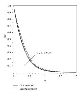
FIGURE 10: Concentration profiles for different values of  $\gamma$  when Nb = Nt = 0.5, Le = 2, Pr = 6.8,  $\sigma$  = -0.1, and *S* = 2.
