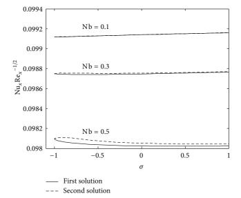
FIGURE 4: Variations of the local Nusselt number (heat transfer rate) with  $\sigma$  for different values of Nb when Nt = 0.5, Le = 2, Pr = 6.8,  $\gamma$  = 0.1, and *S* = 2.
