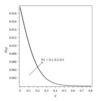
FIGURE 9: Temperature profiles for different values of Nt when Nb = 0.5, Le = 2, Pr = 6.8,  $\gamma$  = 0.1,  $\sigma$  = -0.1, and *S* = 2.
