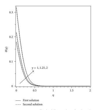
FIGURE 8: Temperature profiles for different values of  $\gamma$  when Nb = Nt = 0.5, Le = 2, Pr = 6.8,  $\sigma$  = -0.1, and *S* = 2.
