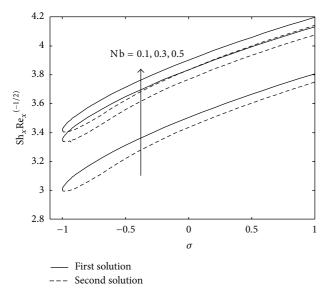
FIGURE 7: Variations of the local Sherwood number (concentration rates) with  $\sigma$  for different values of Nb when Nt = 0.5, Le = 2, Pr = 6.8,  $\gamma$  = 0.1, and *S* = 2.
