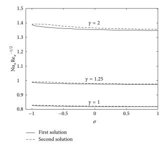
FIGURE 2: Variations of the local Nusselt number (heat transfer rate) with  $\sigma$  for different values of  $\gamma$  when Nb = Nt = 0.5, Le = 2, Pr = 6.8, and *S* = 2.
