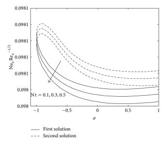
FIGURE 3: Variations of the local Nusselt number (heat transfer rate) with  $\sigma$  for different values of Nt when Nb = 0.5, Le = 2, Pr = 6.8,  $\gamma$  = 0.1, and *S* = 2.
