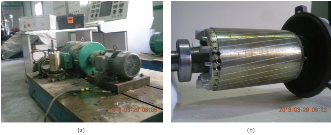
FIGURE 5: Experiment setup to collect motor data and broken rotor used in the tests.
