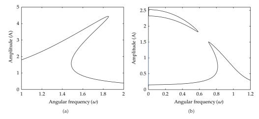
**Figure 3:** The amplitude depending on frequency  $\omega$  for hardening (a) and softening (b) springs.
