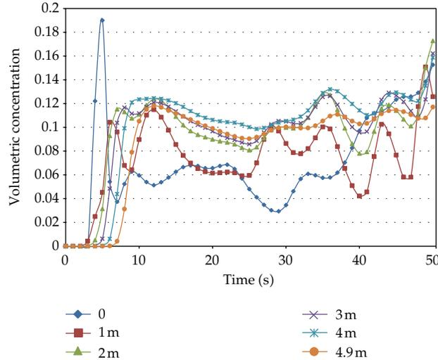
**Figure 10:** Hydrogen volumetric concentration versus time for Model 3 (hydrogen inlet velocity of  $0.67 \text{ m s}^{-1}$ ) at 6 sensor positions, having slip in the  $x$ -direction, and  $C = 0$  at the tunnel exit.
