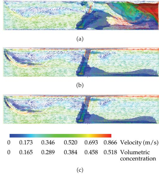
**Figure 8:** Combined velocity vector and isosurface plots for Model 3 at  $t = 55$  s. From top to bottom: boundary conditions as per Section 3 (base settings), slip in the  $x$ -direction, slip in the  $x$ -direction and  $C = 0$  at the tunnel outlet. The colour bar applies to all three figures.
