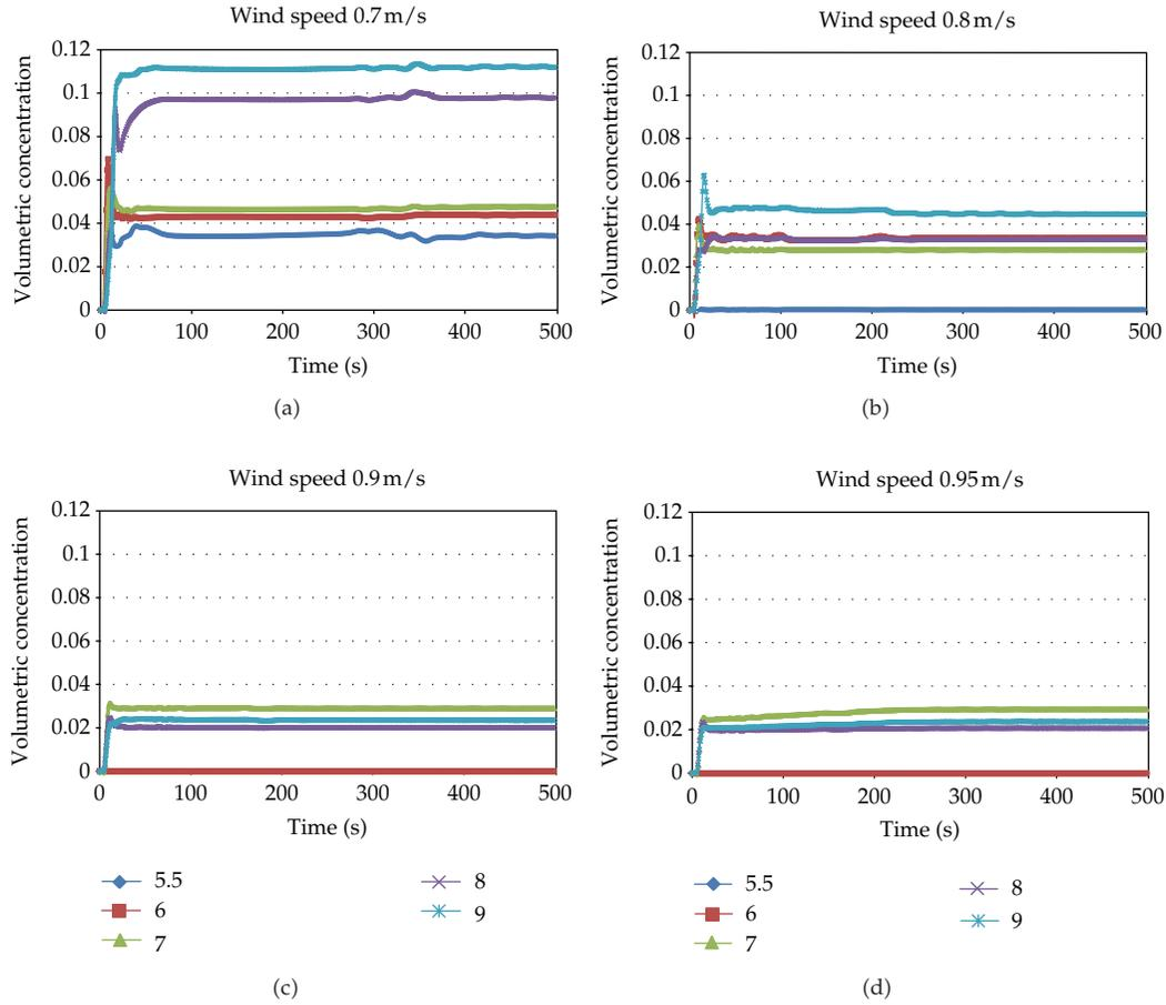
**Figure 7:** Model 2: volumetric concentration versus time for wind speeds 0.7 to 0.95 m s<sup>-1</sup>.
