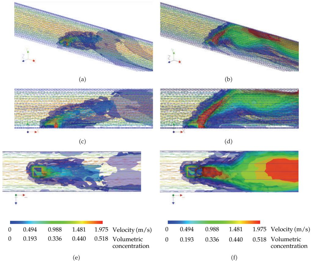
**Figure 6:** Model 1: combined velocity vector and concentration isosurface plots for wind speeds 1.23 (a, c, e) and  $1.235 \text{ m s}^{-1}$  (b, d, f) at 100 s elapsed time. The colour plot applies to all 6 figures. (a, b) Orthogonal view. (c, d) Side view. (e, f) Top (plan) view.
