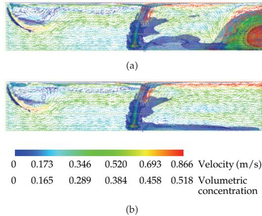
**Figure 9:** Combined velocity vector and isosurface plots for Model 3 at  $t = 127$  s. (a) Slip in the  $x$ -direction, (b) slip in the  $x$ -direction and  $C = 0$  at the tunnel outlet. The colour bar applies both figures.
