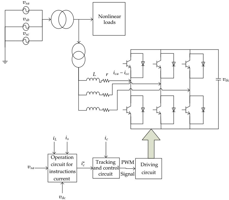
Figure 1: Block diagram for main circuit of APF.
