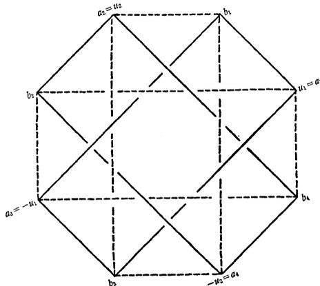
FIGURE 1. Top view of a realization of  $K_{4,4}$  in  $\mathbf{R}^3$  as a tensegrity mechanism. Vertices  $a_i$  are in the plane of the paper, vertices  $b_j$  in a parallel plane above it. Rods are solid, cables dashed.
