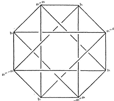
FIGURE 2. Top view of a realization of  $K_{4,4}$  in  $\mathcal{R}^3$  as a framework with two independent degrees of freedom. Vertices  $a_i$  are in the plane of the paper. Vertices  $b_j$  start out in a parallel plane above it, but do not remain coplanar as the mechanism flexes.
