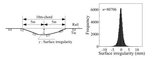
Fig. 2. Surface irregularity. Fig. 3. Distribution of surface irregularities.
