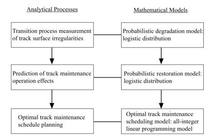
Fig. 1. Flow diagram of the computational procedures.
