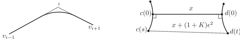
FIGURE 9. On the left, we see the curve constructed from splicing a circular arc of radius \text{MinRad}(v_i) into v_{i-1}v_iv_{i+1} . This curve is C^1 , but not C^2 at the splice points. On the right, we see the setup for Proposition 5-1. On the left and right are arcs c and d with curvature \leq K and length \leq \epsilon . The minimum distance x between them occurs at c(0), d(0) . We prove that this distance is bounded below by the distance between any other pair of points c(s) and d(t) minus (1 + K)\epsilon^2 .
