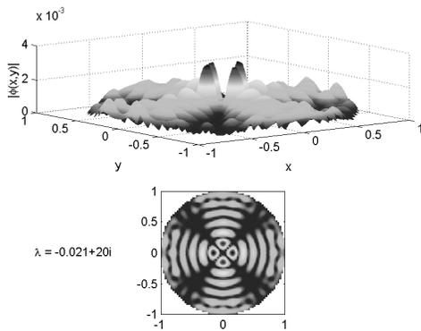
(c) Eigenfunction corresponding to strongly damped eigenvalue  $\lambda = -0.021 + i 20$ .
