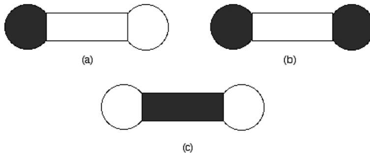
FIGURE 7. Damping geometries for the dog-bone ( $a(x) > 0$  in shaded region): (a) damping in left disc; (b) damping in both discs; (c) damping in shaft.
