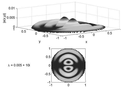
(b) Eigenfunction corresponding to lightly damped eigenvalue  $\lambda = -0.005 + i 10$ .
