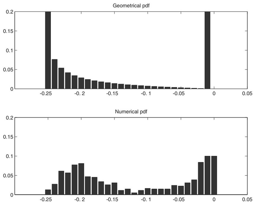
**FIGURE 5.** Probability distribution functions for damping in an interior disc of radius  $r = 0.5$ : comparison of the geometrical and numerically calculated distributions.
