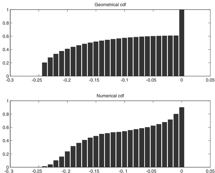
**FIGURE 4.** Cumulative distribution functions for damping in an interior disc of radius  $r = 0.5$ : comparison of the geometrical and numerical calculated distributions.
