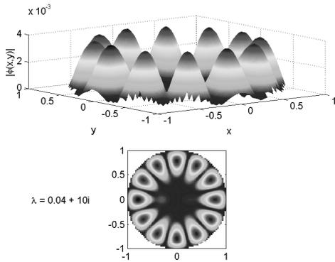
(a) Eigenfunction corresponding to strongly damped eigenvalue  $\lambda = -0.04 + i 10$ .
