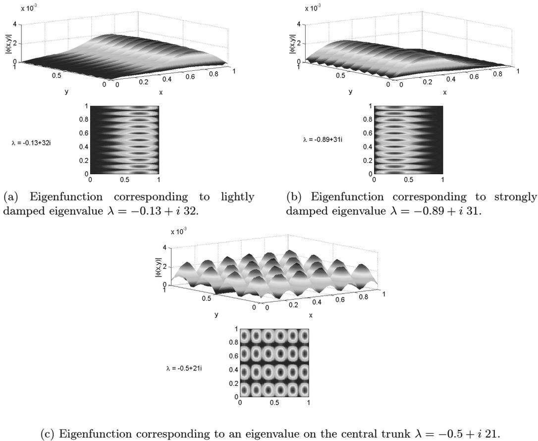
FIGURE 2. Eigenfunctions for damping on the left half of the unit square.
