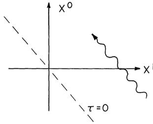
**Fig. 5.** This diagram is meant to illustrate the limitations of a canonical formalism based on light cone coordinates in 1 + 1 dimensions. The dotted line is an “initial value surface”,  $\tau=0$  ( $\tau=(x^0+x^1)/\sqrt{2}$ ). The wave line is a massless particle traveling to the left at the speed of light. Its world path never meets  $\tau=0$ , so its existence cannot be predicted from initial data at  $\tau=0$
