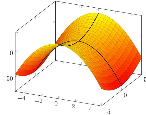
FIGURE 3. Hyperbolic paraboloid.
