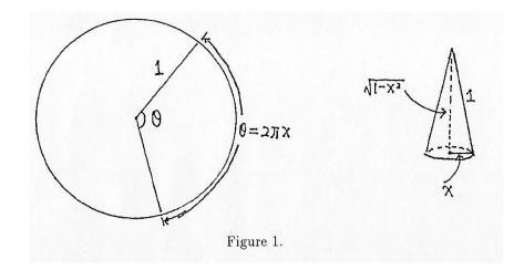
By differentiating V with respect to x we find that V(x) has two critical points 0 and  $\sqrt{2/3}$ . The second derivative test indicates that V(x) attains its maximum at  $\sqrt{2/3}$ , that is,  $V(\sqrt{2/3}) = 2\sqrt{3\pi/27}$ .
