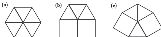
Fig. 1. (a) 3^6 (beehive-shaped) vertex configuration, (b) (4^2, 3^3) (house-shaped) vertex configuration, (c) (3, 4, 3^2, 4) (tent-shaped) vertex configuration
