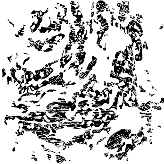
Figure 1. Fractures in 160 m by 160 m granitic rock of the Lac du Bonnet batholith in Manitoba. From Stone et al. (1984). Digitized and post-processed by Professor A.J. Baddeley of the University of Western Australia. The irregular black region is the rock's surface. The white parts represent areas where the rock cannot be observed due to soil, vegetation or water. The white lines through the black regions indicate fractures.
