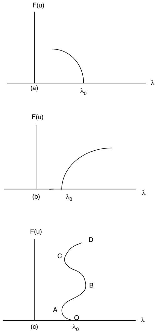
FIGURE 1. Bifurcation diagrams. Figure 1a shows an example of subcritical bifurcation; the branch of nontrivial solutions is unstable. Figure 1b shows an example of supercritical bifurcation; the branch of nontrivial solutions is stable.
